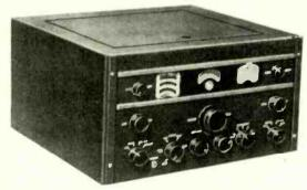
BRAND NEW and in original cases-A.C. mains input. 110V or 250V. Freq. in 6 bands 535 Kc/s-32 Mc/s. Output impedance 2.5-600 ohms. Complete with crystal filter, noise limiter, B.F.O., H.F. tone control, R.F. & A.F. variable controls. Price £87/10/-
