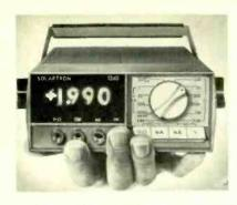
Solartron digital multimeter, type LM1240, which has 26 ranges.
