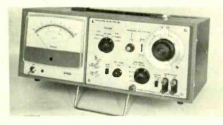
Dymar modulation meter, type 785, for narrow deviation mobile v.h.f. and u.h.f. radio telephone transmissions.
