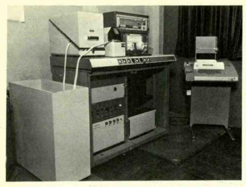
Fig. 10. The Elliott computer installation used in the track-while-scan system. The 920M micro-miniature computer employs a 16k word store.
