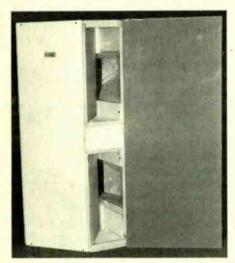
Fig. 5. Two panels of \(\frac{1}{4}\)-in ply complete the compression chamber. The angle formed by the apex of the triangle must of course be \(\geq 90^\circ\) and 9-in wide panels were satisfactory. When one panel has been screwed and glued bracing blocks can be liberally fitted between the internal surfaces of the chamber. The drive unit must be wired up to external terminals. The compression chamber must be airtight.
