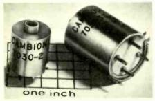
tance range of 12-120mH. Individually the mean inductance values are 15, 22, 33, 47, 68 and 100mH with a variable range of ±20% from the mean. The coils are vertically tuned and have an operating temperature range of -55 to +125°C. Protection from both electrostatic and electromagnetic interference is claimed. Cambion Electronic Products Ltd, Cambion Works, Castleton, near Sheffield.
